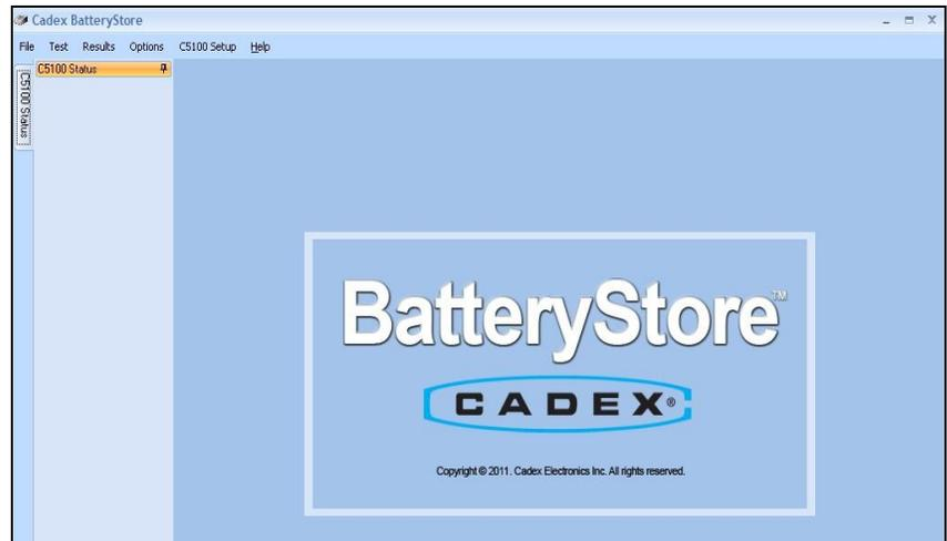
The menu bar on **BatteryStore's Main** window displays six menus: *File*, *Test*, *Results*, *Options*, *C5100 Setup*, and *Help*. Clicking any of these menus displays a list of menu commands.
