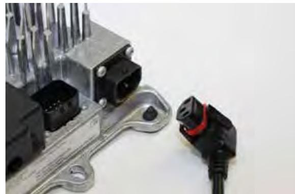
The Delta-Q sealed, locking AC power cable with its red gasket and locking clips.
