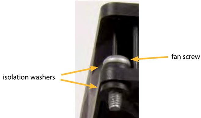
3. Install fan assembly onto charger with fan label down and with leads oriented and routed per illustration.
