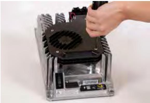
4. With the 4 screws removed, lift up the fan shroud to detach from the charger.
