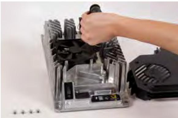
5. Connect fan fastons per illustration. Red wire to positive blade (F+) terminal and black wire to negative (F-) blade terminal. Install rubber strain relief in as shown.
