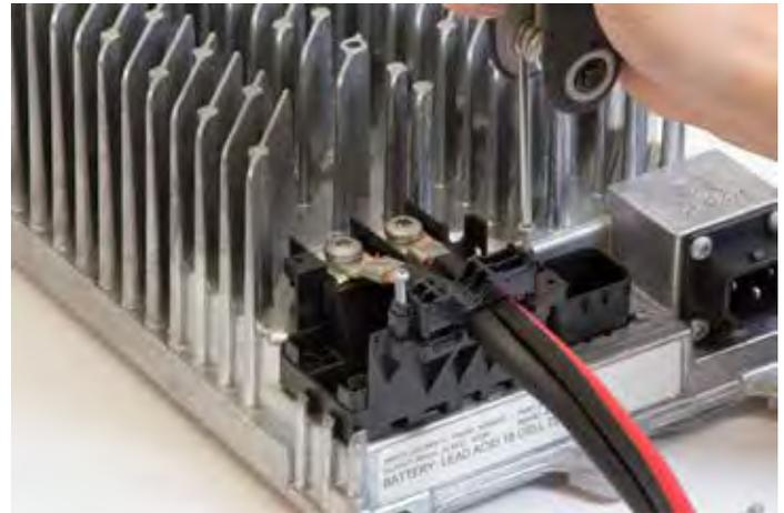
2. Remove the positive and negative battery fasteners (M6 screws). Secure the DC cable in place, fastened with the Torx T30 / M6 screws to a recommended torque of 4.5Nm +/-5%.
