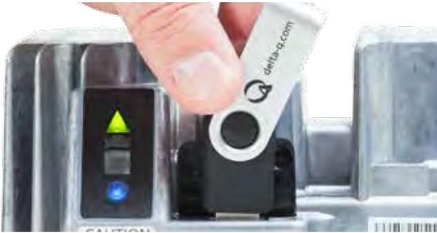
The Universal Serial Bus (USB) host port on an IC Series Charger is used when configuring or retrieving data from the charger.
